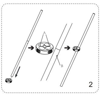
To put the pole through the plastic ring and clip it into position.
